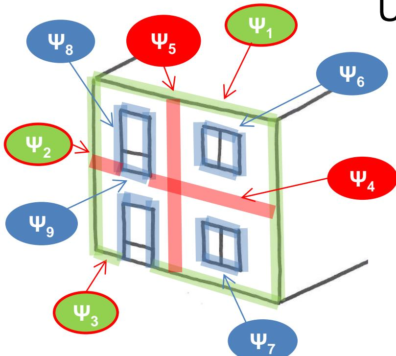
$$U_{\text{progetto}} = \frac{\sum_i (A_i \cdot U_i) + \sum_j (\Psi_j \cdot l_j)}{\sum_i A_i} \leq U_{\text{limite}}$$
